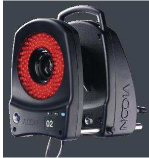
Figure 2.4: The MX3 camera for a Vicon system.
