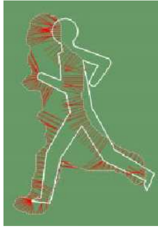
Figure 2.10: Continuous white lines are the contour of the silhouette of the projected 3D model. Dotted white lines are those of the real silhouette. Red lines are the forces necessary to match the contours.
