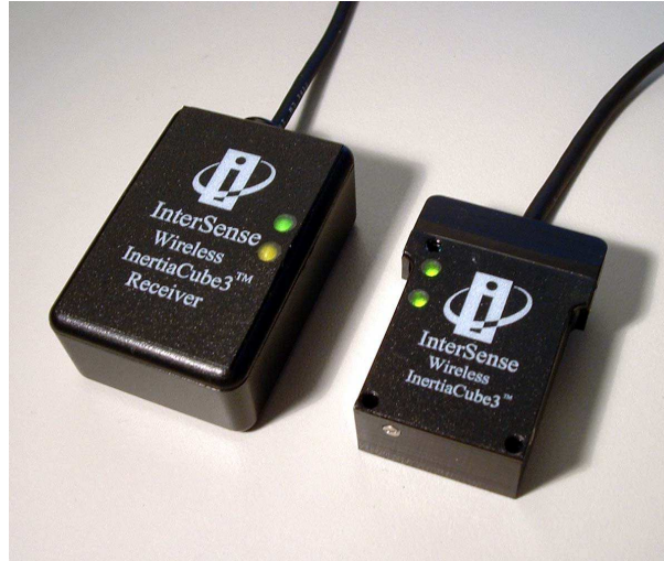
Figure 2.2: Wireless inertiaCube 3: the receiver and the marker..
